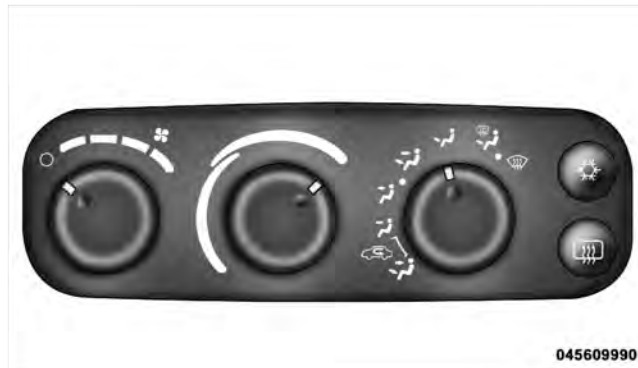
Air Conditioning And Heater Controls
